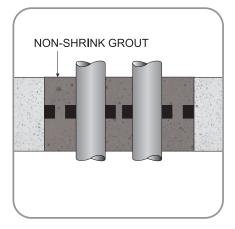
Multiple Pipe Penetrations. Install **Hyperstop DB** around each pipe, as well as, around any block out box construction joint. **Hyperstop DB** 103 shall be installed around penetrationswith less than 4" (100 mm) between penetrations & all polyvinyl chloride(PVC) pipes.
